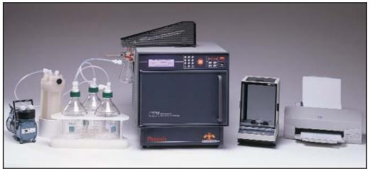
Ash pharmaceutical raw materials, excipients, and finished products in minutes. The system meets ISO 14000 regulations for nitric acid and sulphur dioxide.
