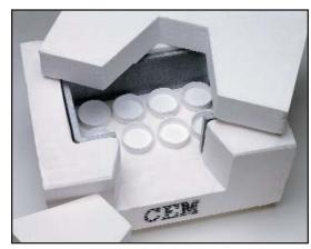
The High Temperature 1200 °C furnace will hold up to 8 (25-mL) crucibles.
